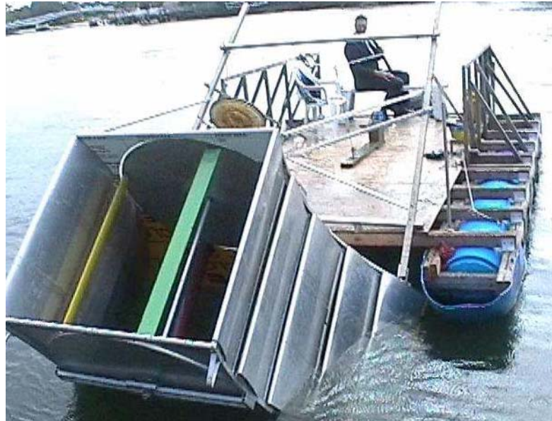
Fig.9. Ducted turbine mounted on motorised barge, lifted partly out of the water to show construction.
