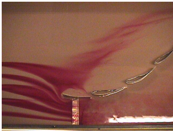
Fig.7. Flow table dye traces showing flow drawn in upstream (on left).
